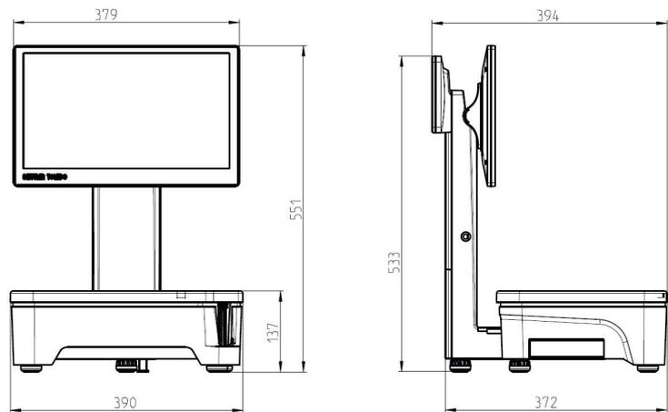
All measurements given in millimeters.
